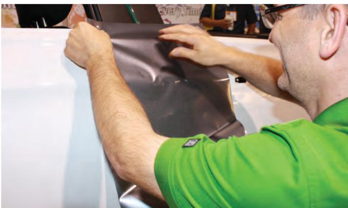
A bridge line can be used to straddle wider gaps on vehicles around doors or the hood.
