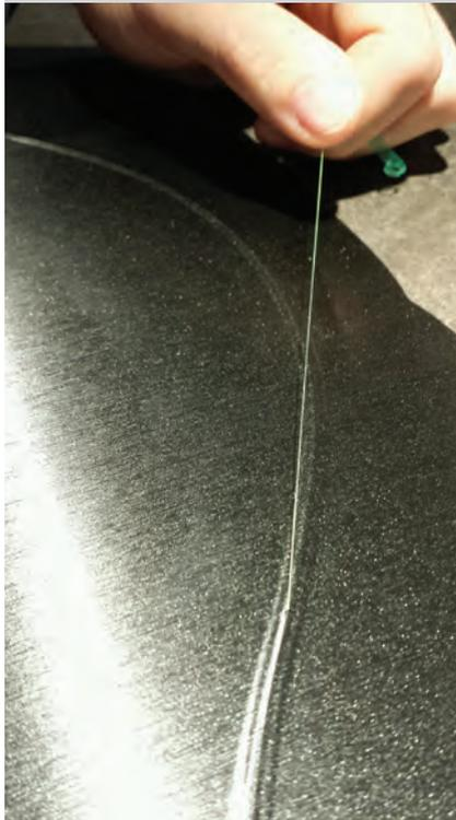
**3** Start the tape and then pull through the vinyl. Keep the filament over top of the tape and low to the substrate to achieve the best results.
